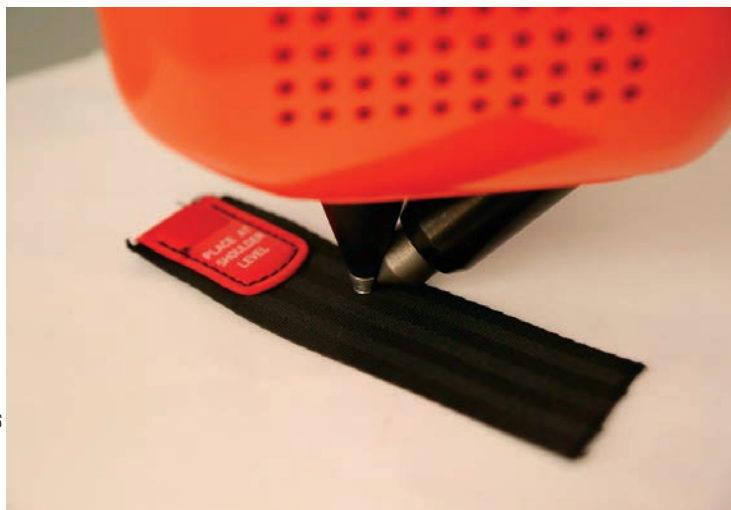
A car seat strap being tested by XRF.
